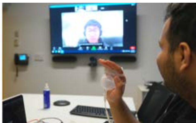
Figure 1: The two application scenarios in which SomaFlatables are used: A: "Pardon": This application consists of bladder placed behind the user's ear which when inflated makes the ear bigger and moves it forward; B: "Bye-Bye": This application consists of the bladder attached to the user's palm which when inflated opens up their hand to signal bye.
