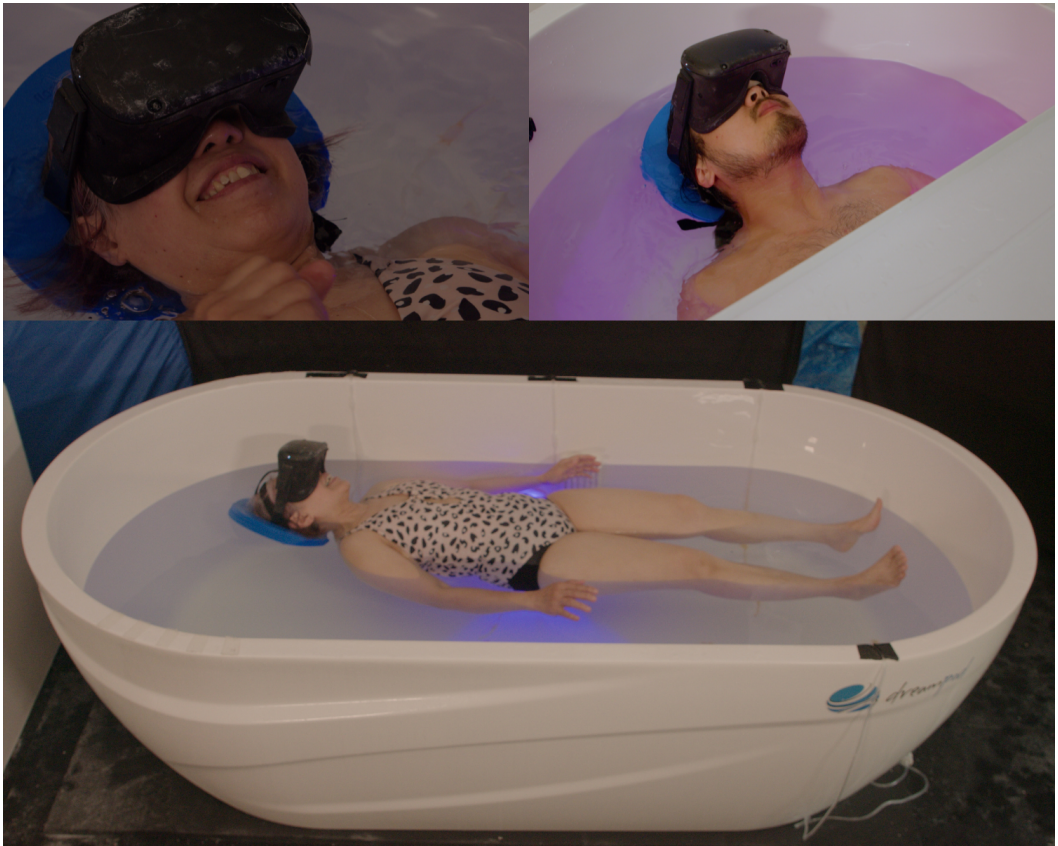
Fig. 1. Participants inside Fluito's floatation tank wearing the heart rate sensor, the virtual reality headset and experiencing Fluito's bubbles delivered through the air pumps' hoses attached to the tank's walls
