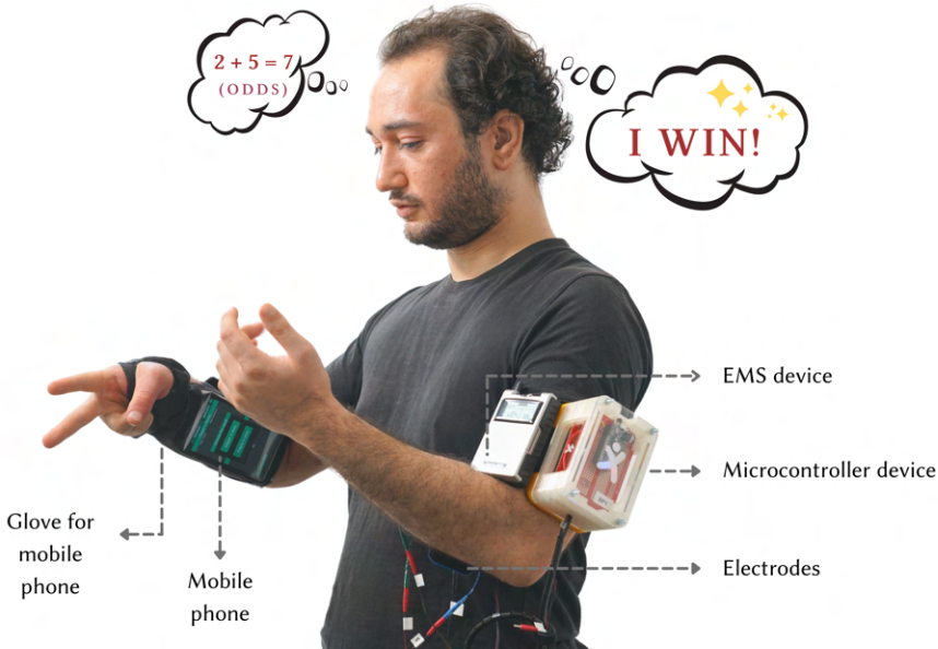
Fig. 3. A participant is wearing the hardware to play “Numbers”. The participant chooses their non-EMS right hand to be “odds”, and the EMS left hand to be “evens”. The with their right non-EMS hand shows a “2”, and their left EMS hand shows a “5” simultaneously, making the sum odd ( 2 + 5 = 7 ). Therefore, the player’s right non-EMS hand wins.
