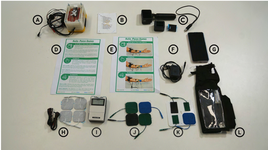
Fig. 2. The EMS assemblage is given to each participant. It contains (A) a microcontroller device, (B) EMS instructions, (C) a GoPro action camera with a spare battery and charger, (D) and (E) game descriptions, (F) a mobile charger, (G) mobile phone, (H) spare electrodes and lead cables, (I) EMS device, (J) and (K) electrodes for the games, and (L) hand glove for the mobile phone.
